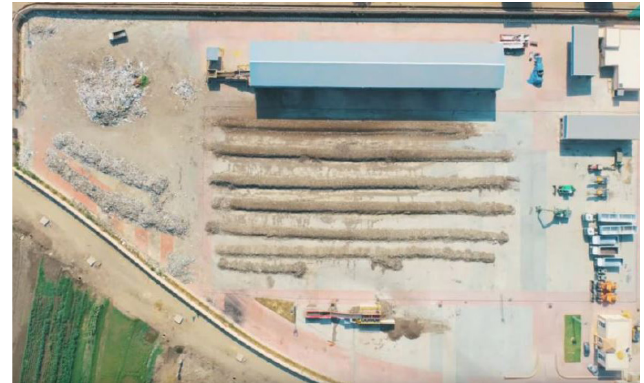
Figure 3: Birdview of MBT in Monufia, Egypt, with mechanical pre-treatment within the hall and open windrow composting. [2]
